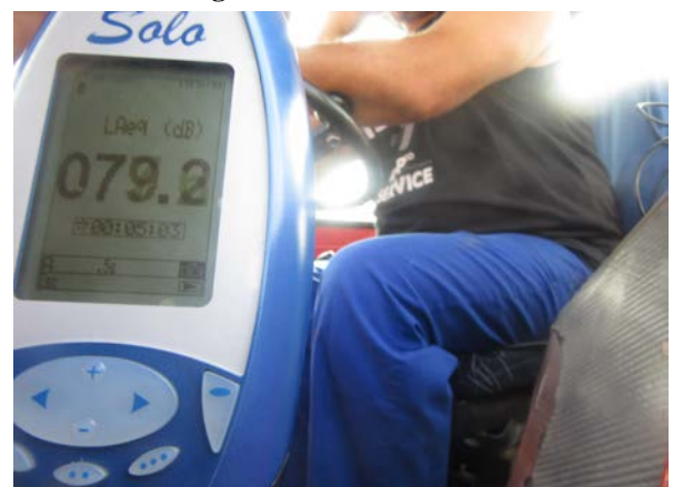
Fig. 8 Noise measurement on the new tractor
