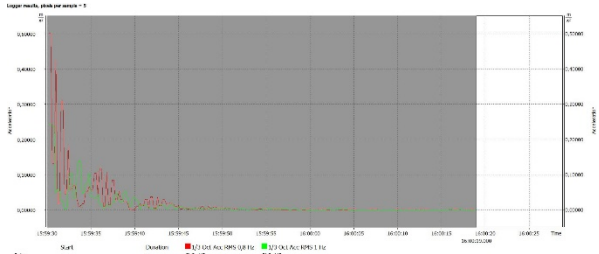
Fig. 5 Logger results graph for compromised measurement for 0,8 Hz and 1 Hz 1/3 octave bands. A characteristic “ski slope” at the beginning of the graph may be seen.
