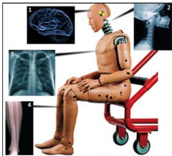
Fig. 5 Hybrid III dummy, doll for vehicle crash tests
