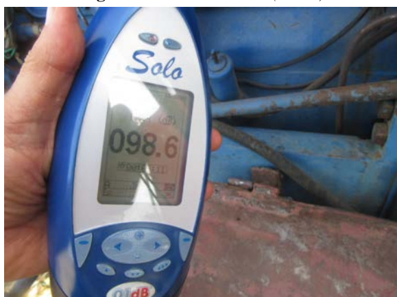
Fig. 7 Noise measurement on the old tractor
