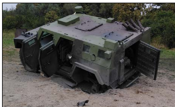
Fig. 9 External appearance of the equivalent of the smaller BOV 4x4 after the explosion
