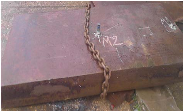
Fig. 3 Measuring points M1 and M2 on armor plate of 3.300 kg mass (dimensions 2 m × 1 m × 0.2 m) set on the support 4×4 (1 m × 1 m × 0.5 m)
