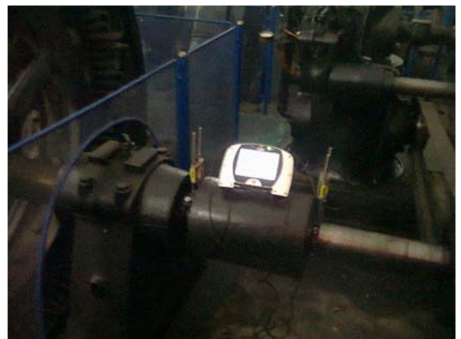
Fig. 4. Adjusting the alignment of aggregate 1 HPP "Sveta Petka"
