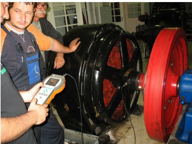
Fig. 7. Vibration analysis of the generator assembly
