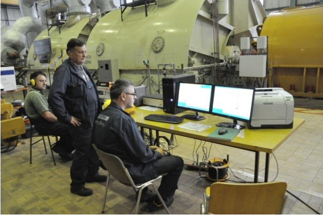
Fig. 7 Vibrometar-VM1 measuring vibrations at turbine-generator set B1-TENT-B (670MW) 12-10-2012.
