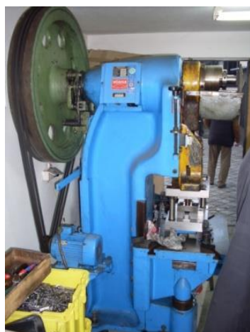
Fig. 1 Eccentric press WÖGTLE (500 KN) and its frequency characteristic at individual operation
