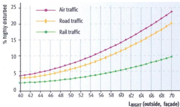
Fig. 3. Percentage noise exposure for various types of transport: air, road and rail
