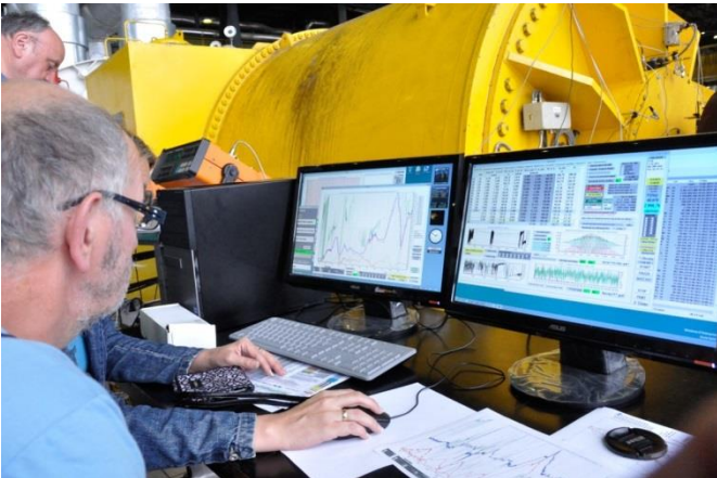
Fig. 8 Vibrometar-VM1 measuring vibrations at turbine-generator set A6-TENT-A (348MW) 13-05-2013.
