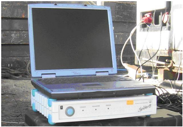
Fig. 8 Measuring device (SPIDER8 connected to a PC)
